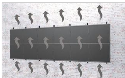
Very good rear ventilation of the modules
