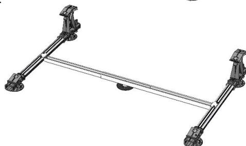
7. Finished. Double check if the anchor bar has washers under and below the anchor bar and there are no gaps between the anchor bar and the Fusion profiles.
