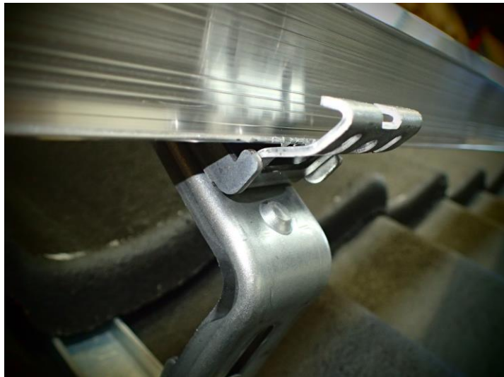
Photo 12 Detail of a mounting rail after it has been broken out of a roof hook (after testing).
