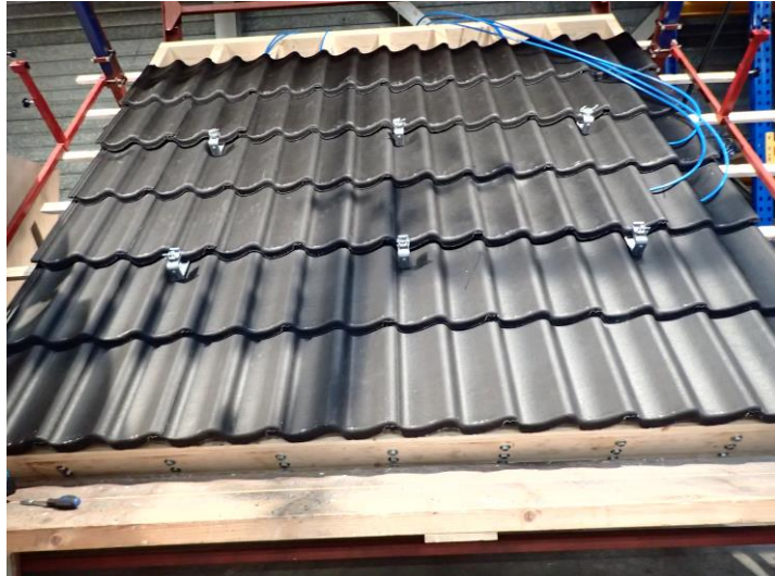
Photo 5 Overview of the system with roof hooks placed in position for a test on PV-modules in portrait layout.
