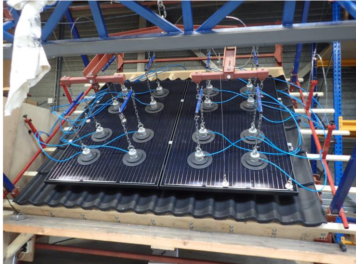
Photo 8 The suction cups are placed in position and the test specimen is ready for testing.
