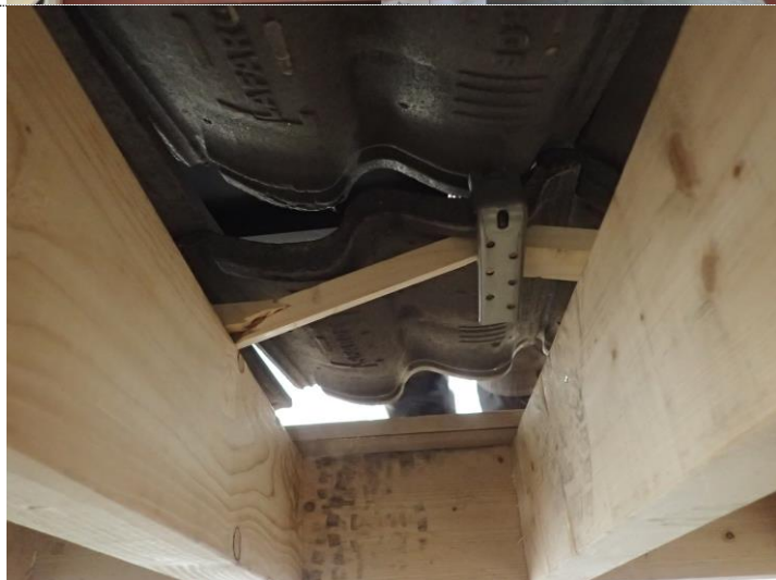
Photo 18 Detail of the breaking of the tile batter at test 3 in landscape layout.
