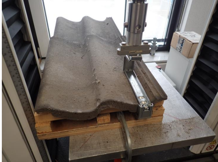
Photo 10 Overview of the test on Sneldek RBB (used), left valley.
