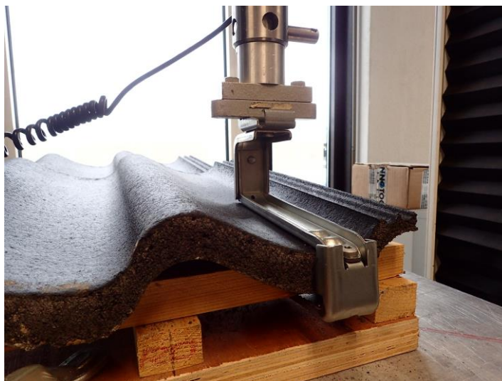
Photo 1 Overview of the test on Sneldek Novo+ (new), left valley.
