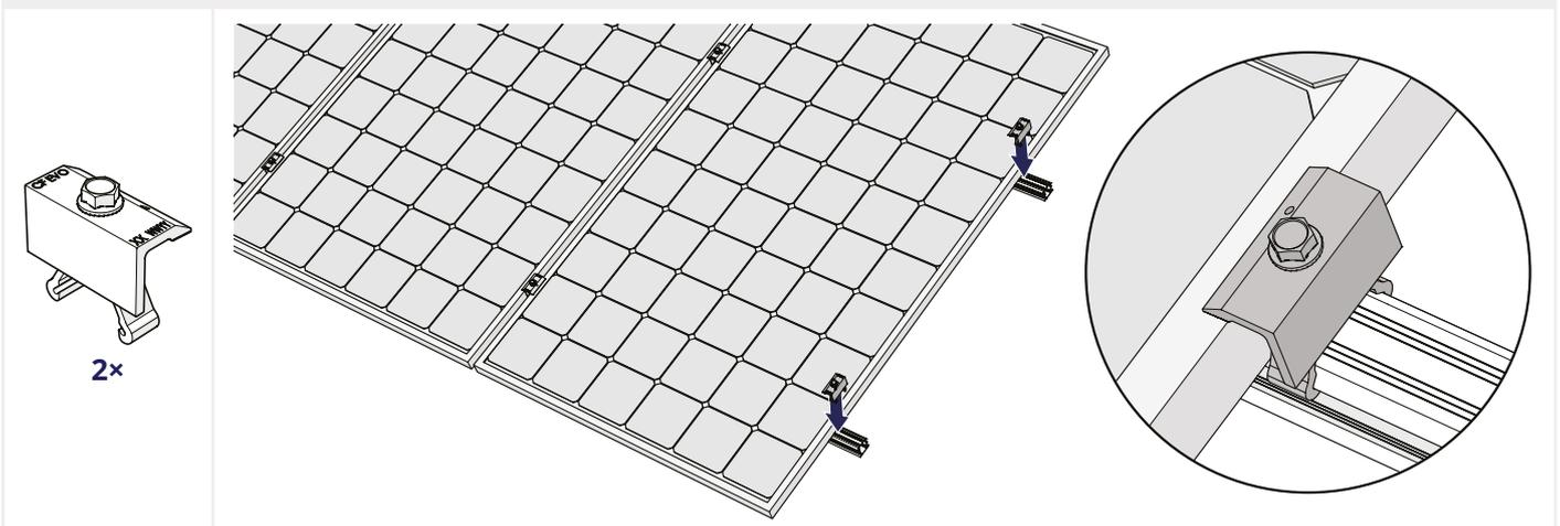
**3 FASTEN THE SCREW OF THE END CLAMPS TO SECURE THE PANEL. APPLY A TORQUE OF 16.5 NM.**
