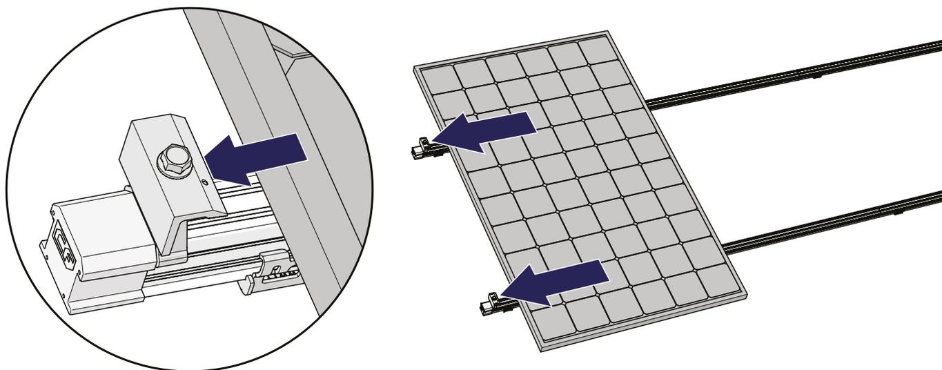
**6 FASTEN THE SCREW OF THE END CLAMPS TO SECURE THE PANEL. APPLY A TORQUE OF 16.5 NM.**
