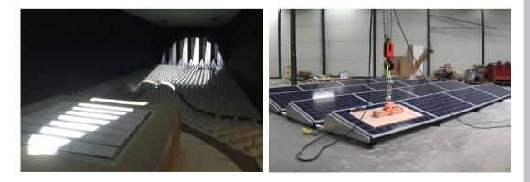
Based on mechanical lift tests carried out by Esdec with improved system connections in the summer of 2021, see right photograph up here, the actual degree of interconnection of the systems was determined and processed by us into the wind tunnel data. These have been
