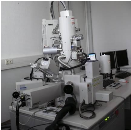
Figure 6: Scanning electron microscope (SEM) Hitachi SU70 for microstructural investigations of the glass surfaces.
