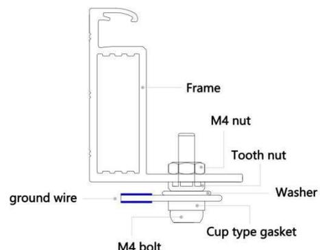
Figure 2. Grounding method
