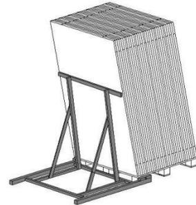
Remove all modules in sequence to complete module unpacking
