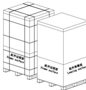
Remove the plastic wrap and wrapping film for the modules to be removed, and remove the cover and packing case
