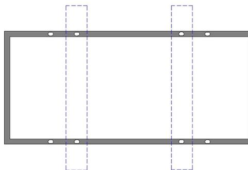
Installation rail vertical to the long side of the module, applicable type:
