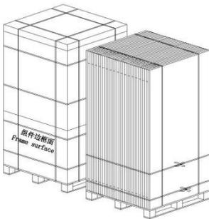
Two people stand on the frame surface of the module to hold the module, while the other person cuts the lower two transverse plastic steel packing belts
