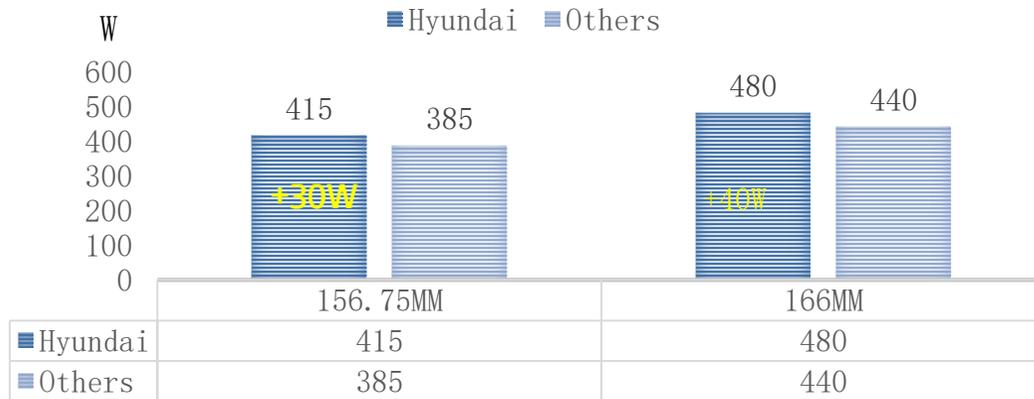
More Shingle modules have higher output per unit. For the same installation capacity, 8% less field is utilized
