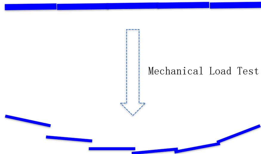
Mechanical load test: with shingled flexible cell joints and absence of metal ribbon, the shingle cell string handles load well---the flexible adhesive acts as a shock buffer and absorbs bending energy. In comparison the ribbon soldering joints of conventional cell strings develop cell cracks easily under external load.
