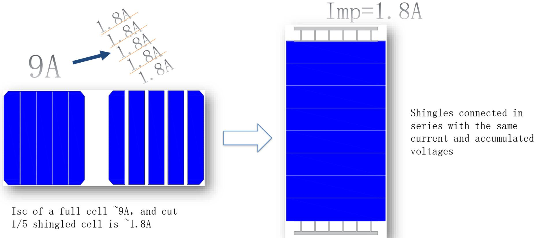
Isc of a full cell  $\sim 9A$ , and cut
