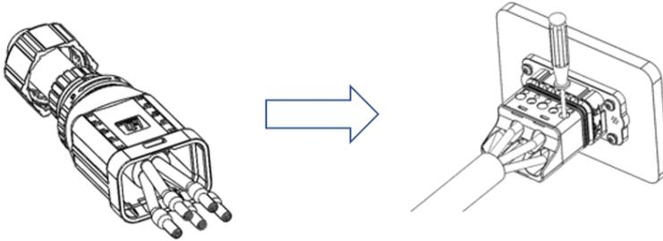
4. Insert the main body into the rubber core and hear the "click" sound.
