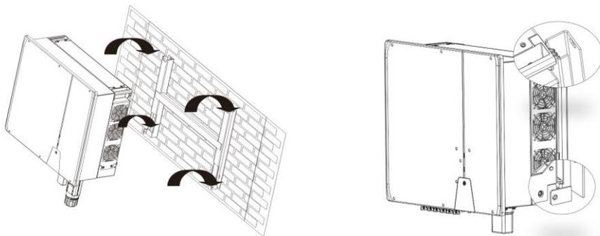
4. Secure the inverter to the mounting bracket on both sides using two M5 screws. Screwdriver type:PH2, torque:2.5Nm.
