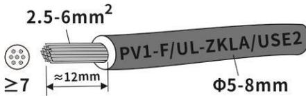
2. Route the stripped cable all the way into the DC connector. Ensure that the stripped cable and the DC connector have the same polarity.
