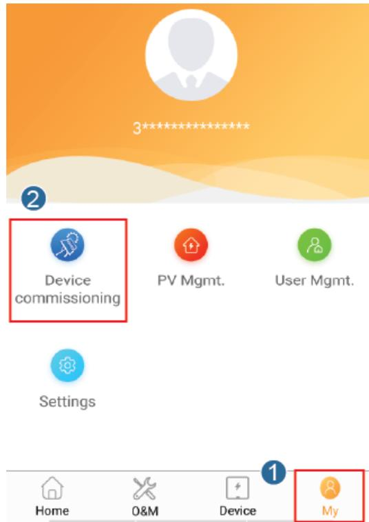
**Step 2** Connect to the inverter WLAN. Log in as **installer**, and perform **Quick settings**.
