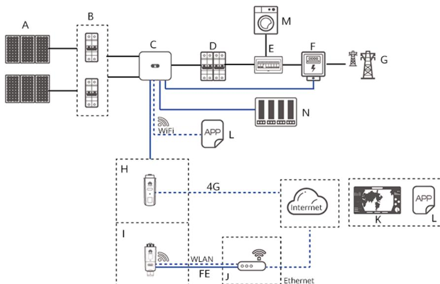
**Figure 2-3** Networking application - Inverter cascading scenario (optional in dashed boxes)
