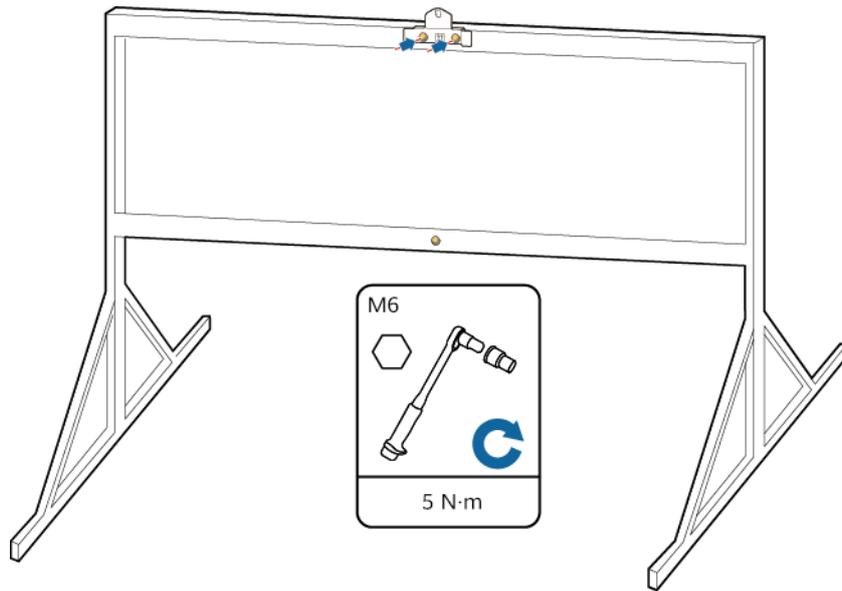
**Step 4** Install the SUN2000 onto the mounting bracket.
