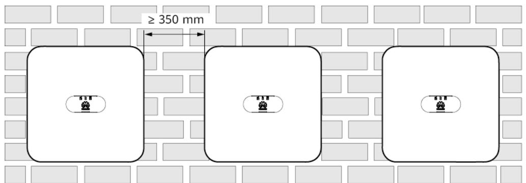
**Figure 4-4** Staggered installation (recommended)
