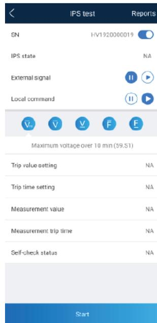
**Step 2** Choose to start the S1 or S2 check as required. The default check type is S2. To start the S2 check, you need to set **External Signal** or **Local Command**.
