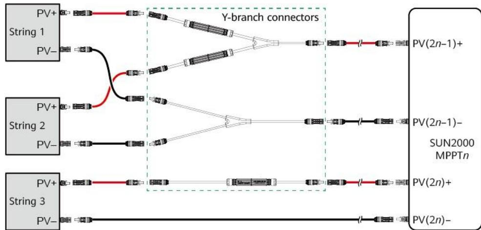
**Figure 5-13** Connecting Y-branch connectors to the solar inverter with a safe distance (recommended)
