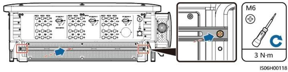
**Step 2** Bind the Y-branch connectors on the beam.
