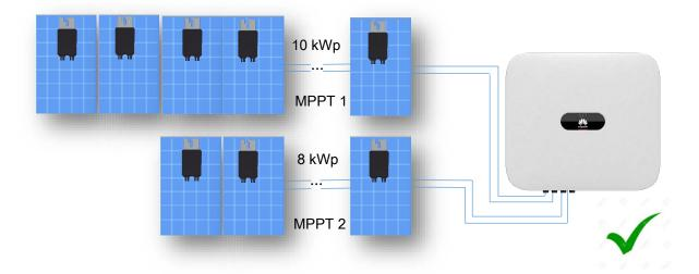
• If total PV module power capacity is higher than 20KWp, keep 10KWp PV modules connect to only one string of the first MPPT tracker. Then split the rest PV modules into
