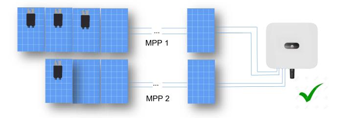
2. For SUN2000-12/15/17/20KTL-M1 inverter, inverter has two MPPT trackers and each tracker has two string input connected in parallel.
