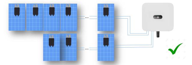
2) For SUN2000-12/15/17/20KTL-M2 inverter, it has two MPPT trackers and each tracker has two string inputs connected in parallel. Full optimizer deployment has following restriction when connecting PV modules to both string inputs of each MPPT tracker:
