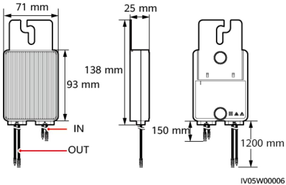
Figure 2-4 SUN2000-450W-P2/SUN2000-600W-P (short input power cable) dimensions
