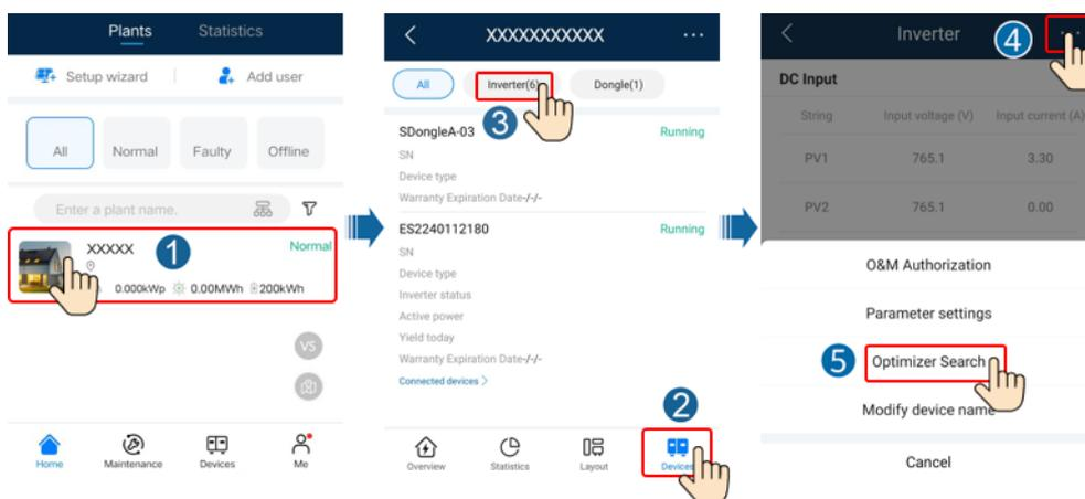
**Step 7** Choose **Devices > Connected devices > Optimizer**, tap **Optimizer No.**, select the faulty optimizer, tap **Device Replacement**, and replace the optimizer as prompted.
