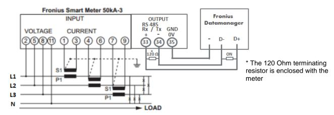
Current transducers with a secondary current of 1A and 5A can be used.
