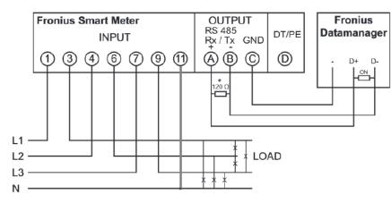
\* The 120 Ohm terminating resistor is enclosed with the meter
