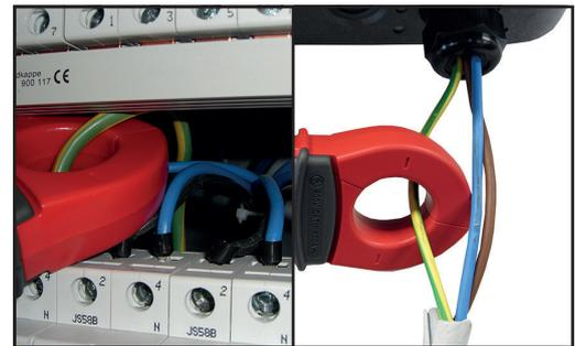
Examples of measuring the ground conductor current
