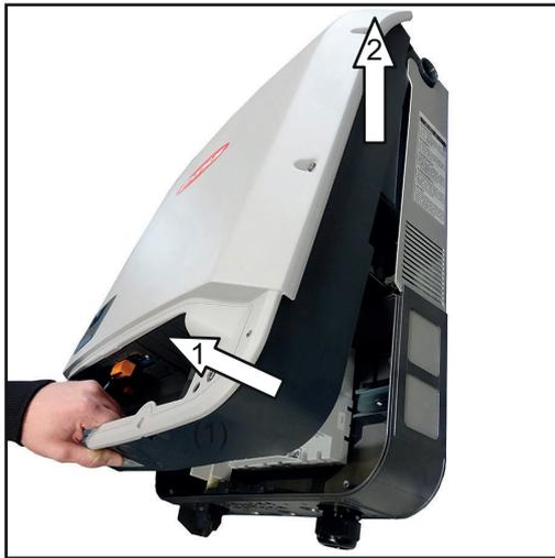
**NOTE!** To avoid damaging the base shell, do not angle the inverter by more than 11°.
