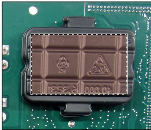
**NOTE!** Do not press on the marked area -> this will damage the PCM material
