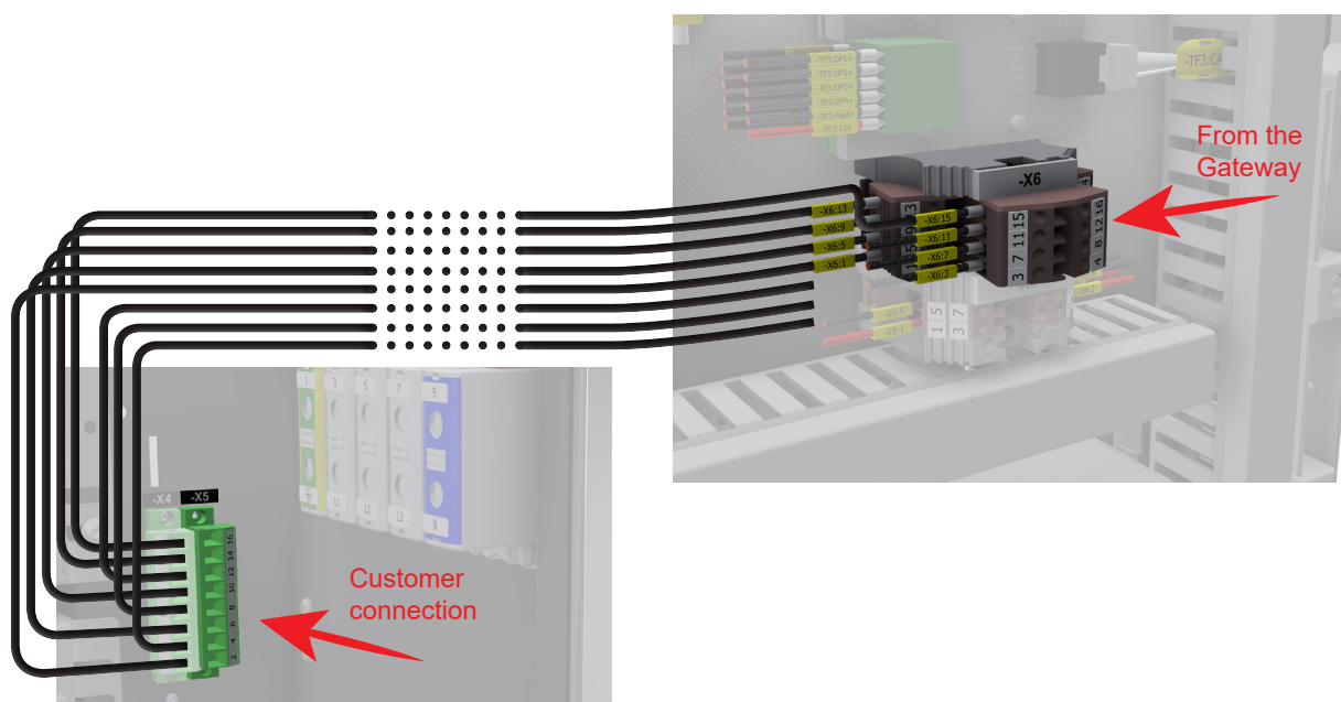
Figure 4.22 Customer spare terminals connection
