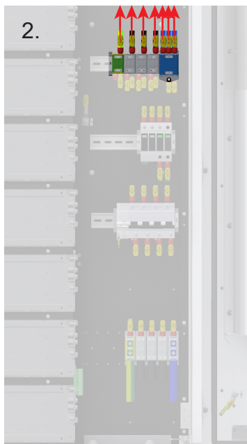
Figure 4.4 Disconnecting cables from terminals -X2
