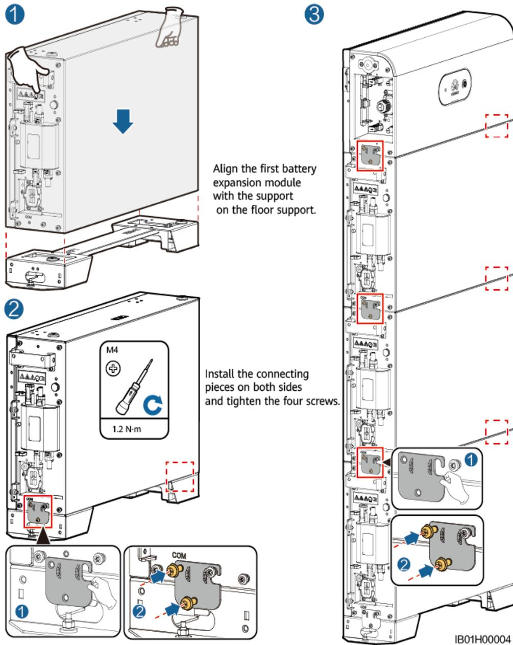
Align the first battery expansion module with the support on the floor support.
