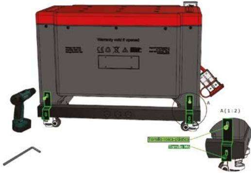
d) When mounting TWO modules, the front of the modules have to be fastened together using the fastening plates (long flat) and screws that are supplied with each of the modules. An ALLEN key is required.
