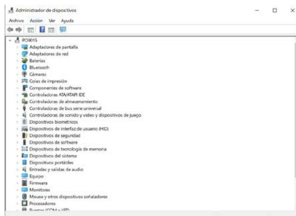
3. Open the “Ports (COM and LPT)” path and note down the COM value (in this case COM13) for subsequent use in the PuTTY program
