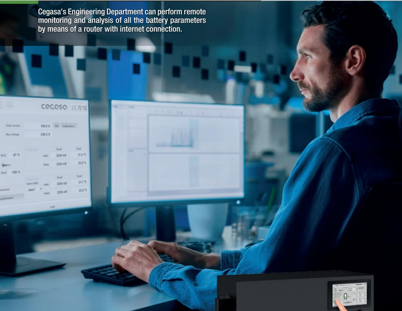
Cegasa has developed user-friendly software that enables in-situ display of all the parameters provided by the BMS on a 7-inch touchscreen:
